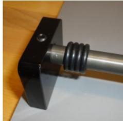
Center Slide Bar and tighten both set screws. Side bumpers to the support. It should look like the image to the right.
