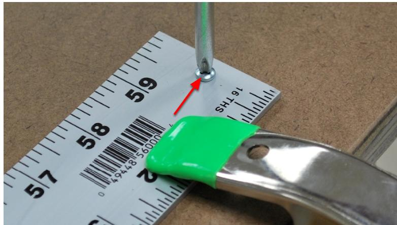
Insert and tighten one screw on the end, and recheck alignment. If alignment is good, fasten the other end. Check alignment again. If alignment is good, fasten the rest of the ruler. Once the ruler is installed, you are ready to use your Studio glass cutter.
