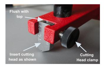
Insert cutting head into slot and tighten cutting head clamp. The top of cutting head should be flush with top of slot.
