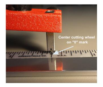
When the cutting head is replaced, the centering may need to be adjusted.
